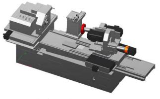
Examples of configurations of the grinding spindle revolver with vector disk and belt-driven spindle
