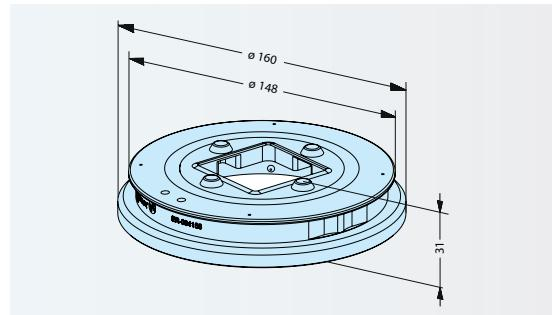
**ER-094112 Dichtring ITS50 C für SSF manuell**
